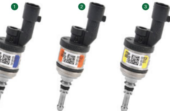
Gas flows from the rail to the bottom of the injector, then it is injected into the intake manifold when the electromagnet moves the shutter to open the passage.
